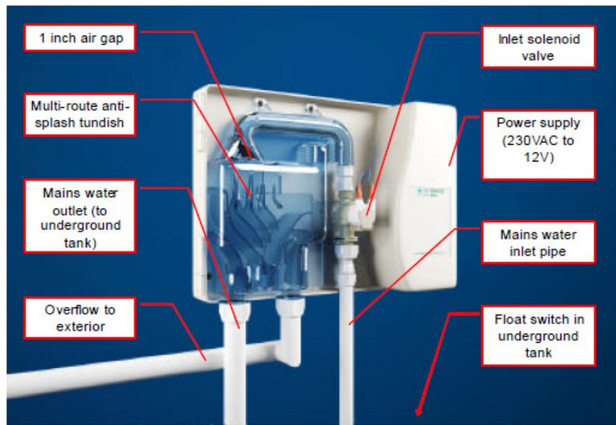
appliances going. The principle for a direct feed system is simple; a float switch detects when the rainwater storage tank is empty and opens an electrically-actuated solenoid valve so that mains water flows into the bottom of the tank. When the float switch floats off the bottom of the tank it closes the solenoid valve. The bulk of the storage tank remains empty ready to admit the water from the next rain shower.
